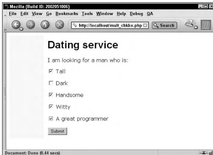
Figure 17-5: A cluster of check boxes
