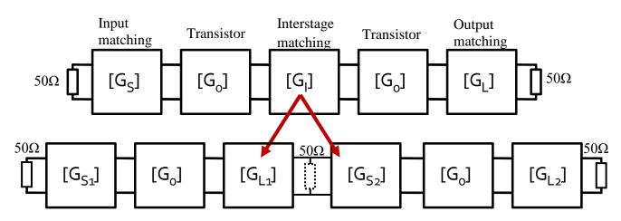
For the design of the matching networks we will use the method of getting a required reflection coefficient ( $\Gamma_S$ ,  $\Gamma_L$ ) using a series transmission line and a shunt stub, starting from the 50 $\Omega$  source/load, see L7/2021, S128-140, S165-169.
