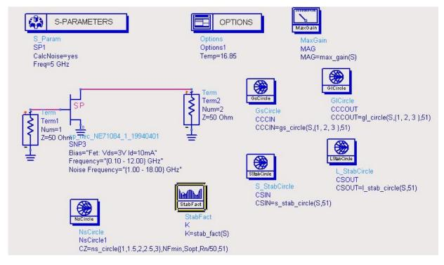
If you don't use ADS to compute the gains available by matching the input/output port of the transistor, then this calculation must be performed manually, those values being necessary to be able to instruct ADS to display the required circles (remember that the circles you request – values between the curly braces {} – depend on the available gains/noise figure for your particular transistor). The modulus of the required S parameters can be very easily read from the S parameter file for 5GHz.
