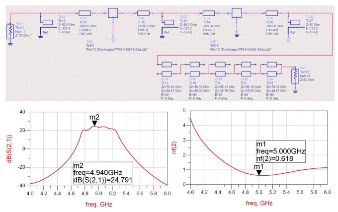
The only problem with the final schematic is that at low frequencies at the end of the passband (~4.75GHz) we have a decrease of the gain. This can be compensated by a final adjustment of the transmission lines, preferably with the adjustment of the line in the interstage matching network, whose adjustment altered the noise factor.
