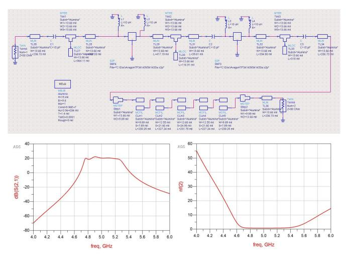
For the sample assignment inserting the biasing components in the schematic decreases the gain below the minimum gain condition of 20dB in a restricted frequency range. A final adjustment/optimization of the schematic provides the fulfillment of this criterion.
