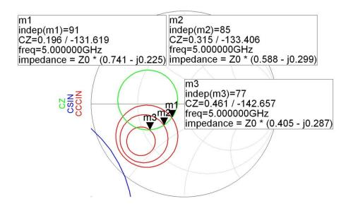
We will be able to choose the position indicated by the marker m3  $(0.461\angle -142.66^{\circ})$  for which we obtain the solution listed below. If we later encounter stability problems we can try to improve it by choosing another point (for example m1, farther from the stability circle but a gain reduced by 1dB).
