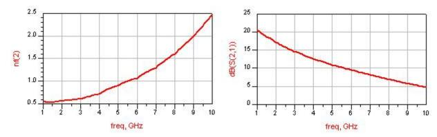
For the sample assignment, we can start from information from the selection guide/datasheet, so from NF = 0.5dB, G = 17.5dB at 2GHz, we can estimate a performance of about NF =  $0.7 \div 0.8dB$  and G =  $14 \div 15dB$  at 5GHz, at 4V/60mA bias.
