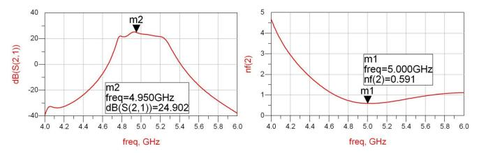
After the final tune, a slightly better noise factor is obtained (F = 0.591dB) and a power gain with a ripple of approximately 3dB in the bandwidth, between 4.75GHz and 5.25GHz, with a minimum of 21.6dB and a maximum of 24.9dB.
