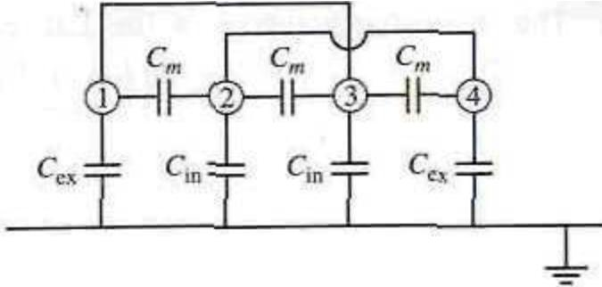
$$C_{in} = C_{ex} - \frac{C_{ex}C_m}{C_{ex} + C_m}$$
