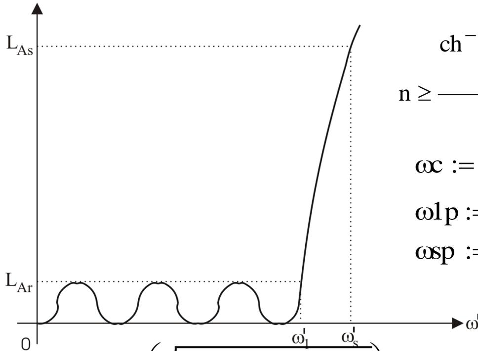
$$n \geq \frac{\text{ch}^{-1} \left( \sqrt{ \left\{ \left[ \left( 10^{0.1 L_{As}} \right) - 1 \right] / \left[ \left( 10^{0.1 L_{Ar}} \right) - 1 \right] \right\} } \right)}{\text{ch}^{-1}(\omega'_s / \omega'_1)}$$
