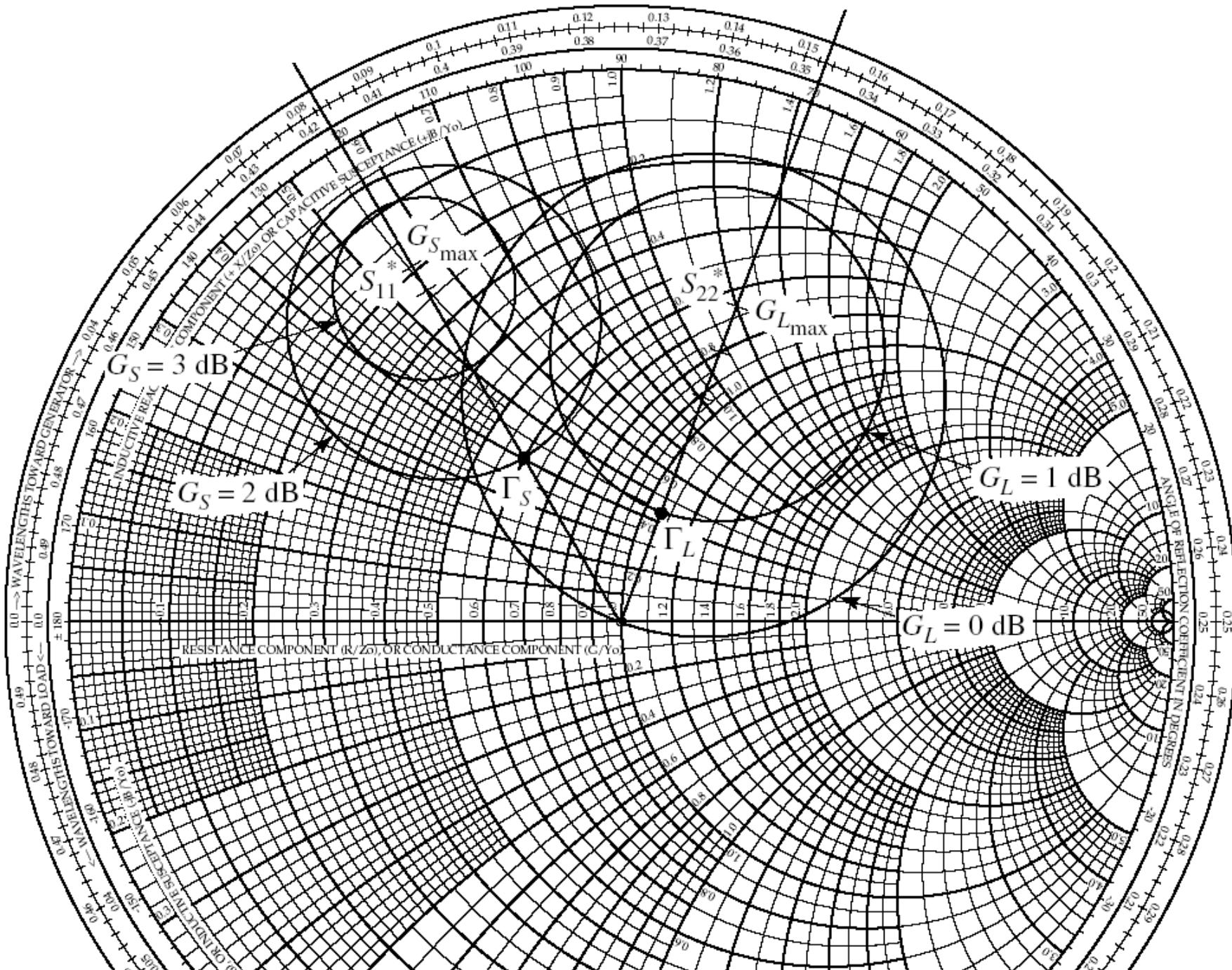
$$\Gamma_S = (C_S(G_{S2}) - R_S(G_{S2})) \cdot e^{j \cdot \arg(C_S(G_{S2}))} = 0.336 \angle 120^\circ$$
