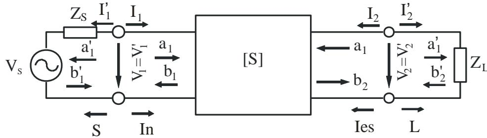
$$G = \frac{P_L}{P_{in}} = \frac{|S_{21}|^2 (1 - |\Gamma_L|^2)}{\left(1 - |\Gamma_{in}|^2\right) |1 - S_{22}\Gamma_L|^2}$$
