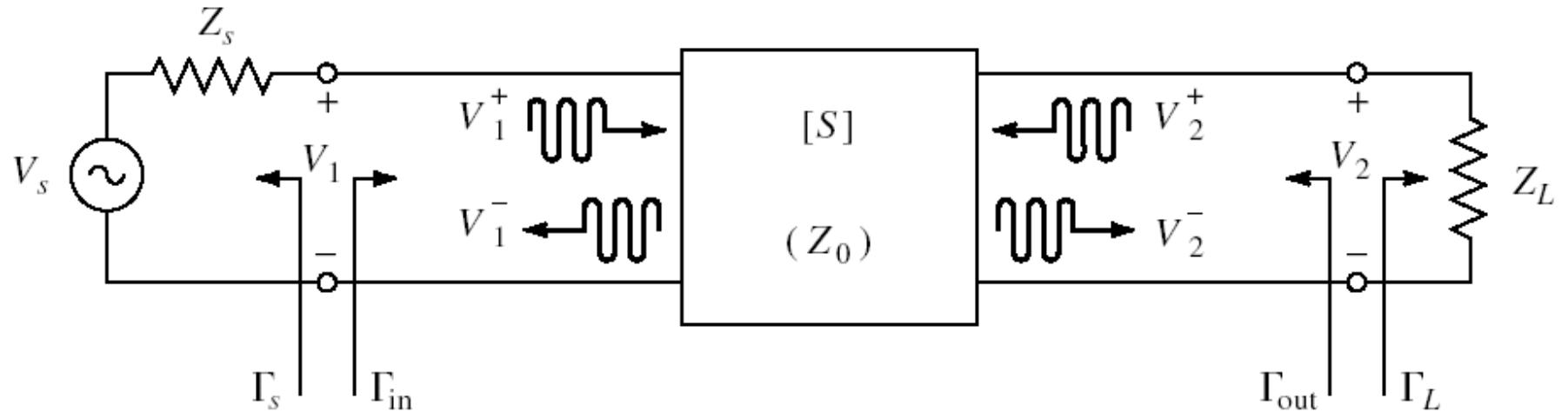
$$V_1^- = S_{11}V_1^+ + S_{12}V_2^+ = S_{11}V_1^+ + S_{12}\Gamma_L V_2^-,$$
